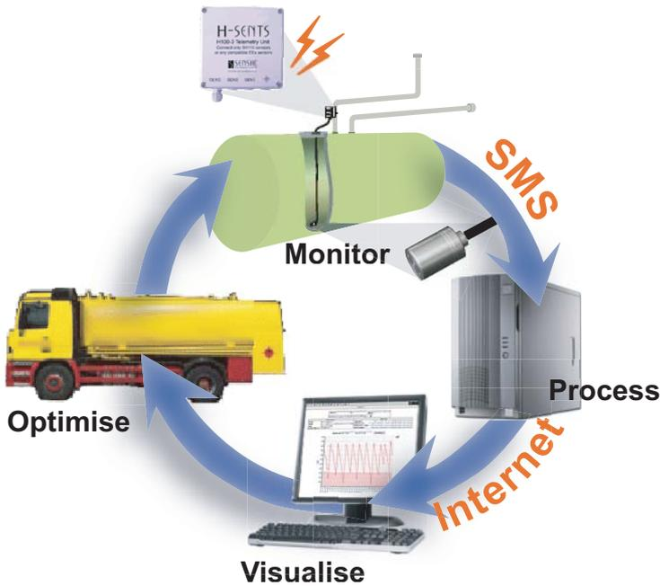
An easily installed GSM-based system to monitor tank levels via the internet.
